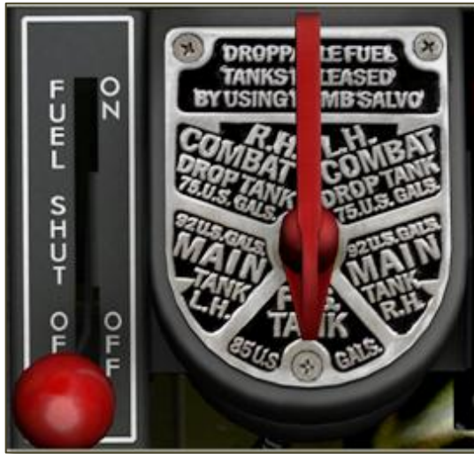
Figure 18: Fuel Selector Valve
