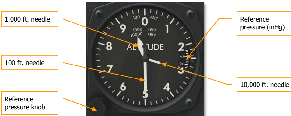
Figure 44: AN5760-2 Pressure Altimeter indicating 29,500 ft.
