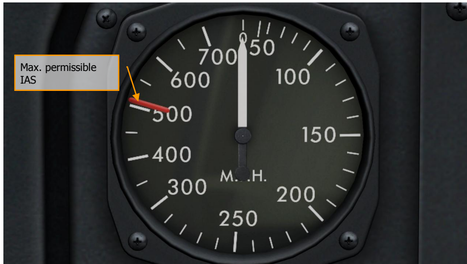
Figure 85: Max. permissible IAS 505 mph (808 km/h, 440 knots)
