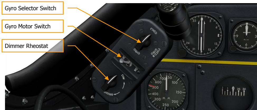
Figure 37: K-14 gunsight selector-dimmer panel
