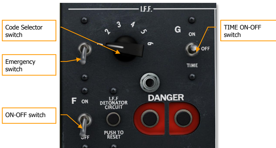
Figure 77: SCR-695-A IFF Radio
