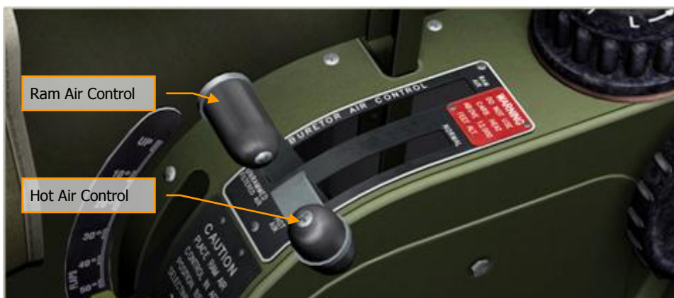
Figure 67: Carburetor Air Controls
