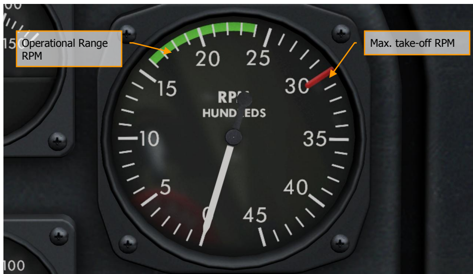
Figure 84: Max. take-off RPM 3000. Operating Range 1600...2400.
