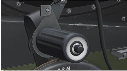
Figure 94: Throttle Control handle with twist grip
