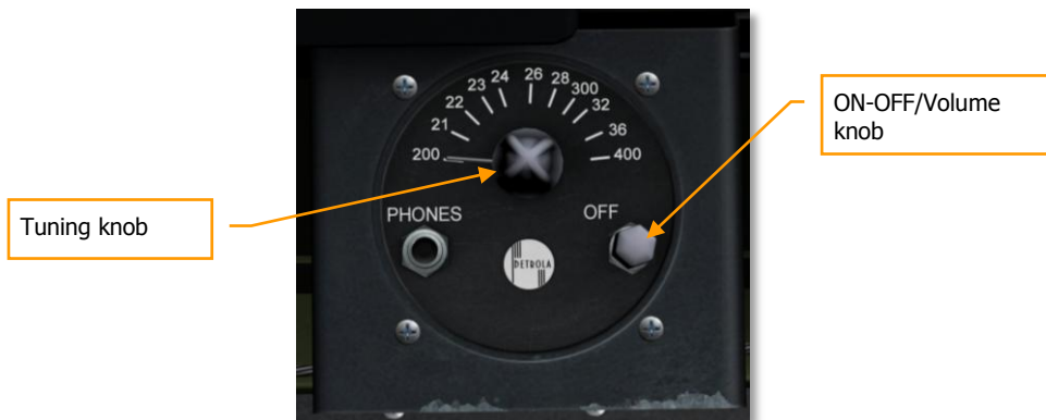
Figure 79: BC-1206 "Detrola" Radio Range Receiver
