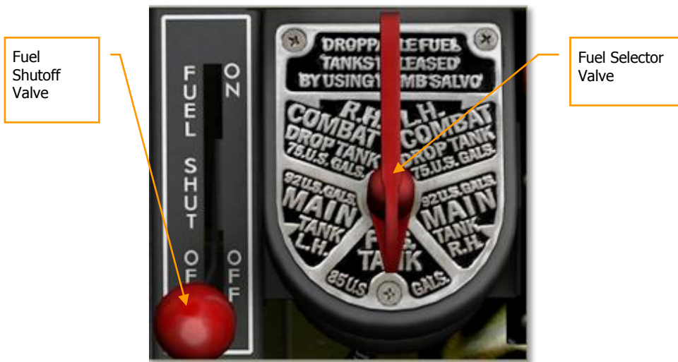
Figure 60: Fuel Shutoff and Selector Valves
